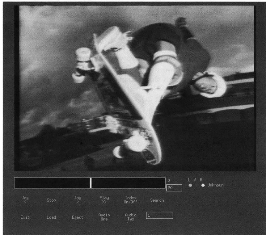
Figure 19.4 A Galatea client application. This is a video controller called “gctl” distributed with the Galatea software. The custom spring-loaded scrollbar affects the rate of playback of the current video device. The middle position pauses the device, while positions to the left and right cause it to speed up in forward and reverse. This was designed to emulate the physical “joystick” controllers found in many commercial video editing systems. There is also a set of indicator “lights” showing the currently selected channels (video, left audio, and right audio) and a list of available video volumes (if more than one is present).
