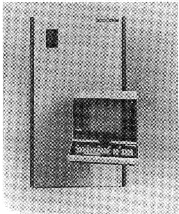
The CC-85 from Computer Communications, Inc. is designed for controlling a high-volume data communications network of IBM and IBM-compatible mainframes. Peripherals include a micro-processor-controlled color CRT console that is used as a system supervisor, system monitor, or engineering console. The CC-85 can support up to seven channel-attachable host computers and up to 1232 communications lines of mixed speeds and protocols.
